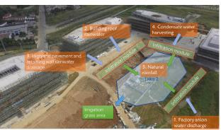
The proposed project will construct 2 artificial lakes with over 15,000 m<sup>2</sup>. STAR water will integrate the biofiltration technology for the stormwater collection, filtration and reuse for the lake water supply. Additionally, STAR Water will introduce a vegetated biofiltration system for landscaping design.
