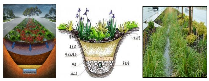
Bio-swale system on Lougheed Highway, Canada was constructed in 2009. Bio-swale system is located in the median strip of highway, which collected and treat highway road surface runoff to remove pollutants such as heavy metals, PAHs, hydrocarbons, and TSS etc. This vegetated biofiltration system also reduces flooding risk and heat from the road, and treated stormwater can be dischaged to environment safely.
